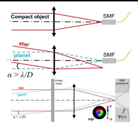
Single-object spectroscopy (e.g. PRV, transits) at high-angular resolution: SMF suppresses modal noise and sky background/OH lines by 2 orders of magnitude
